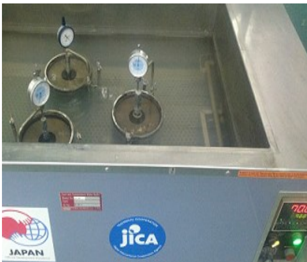
Fig 2. Test to determine the volume expansion of steel slag aggregates
