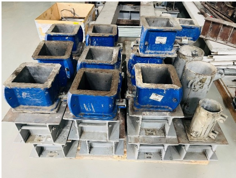
Fig. 12. Cube mold for compressive strength testing
