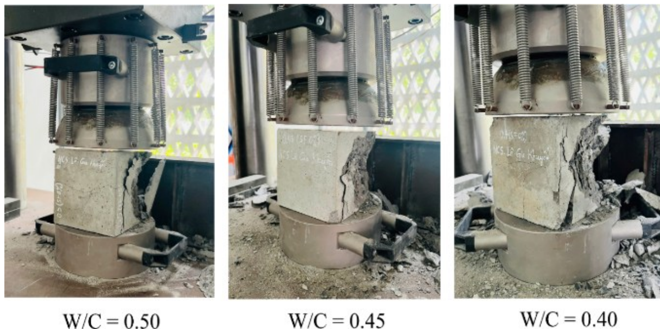
Fig. 14. Compression failure test specimen
