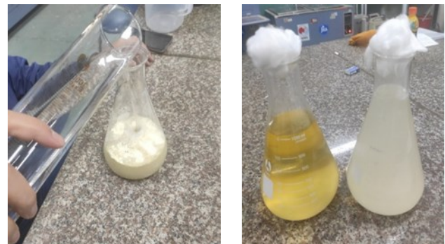
Fig 5. Experiment on mixing and precipitation of calcium carbonate of two microbial preparations bacillus subtilis in a mixture of nutrient medium type 1
