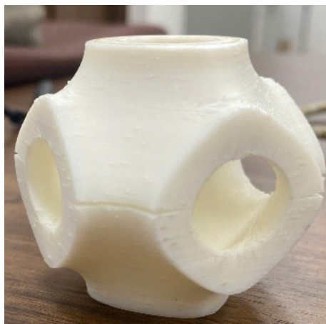
Fig. 7. Illustration of primitive sample fabricated with PLA material
