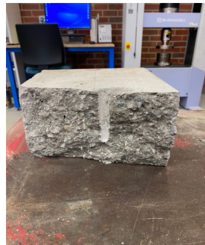
Fig. 6. Representative Pull-out Failure (B4-48-90)
