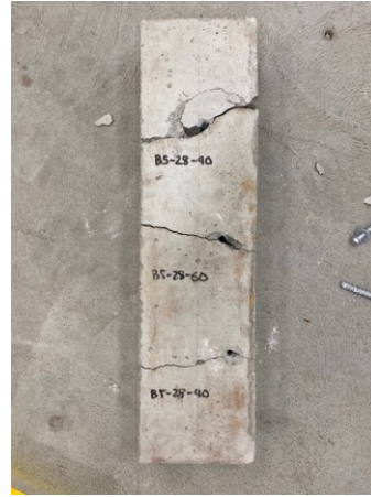
Fig. 8. Specimen Demonstrating Splitting Failure
