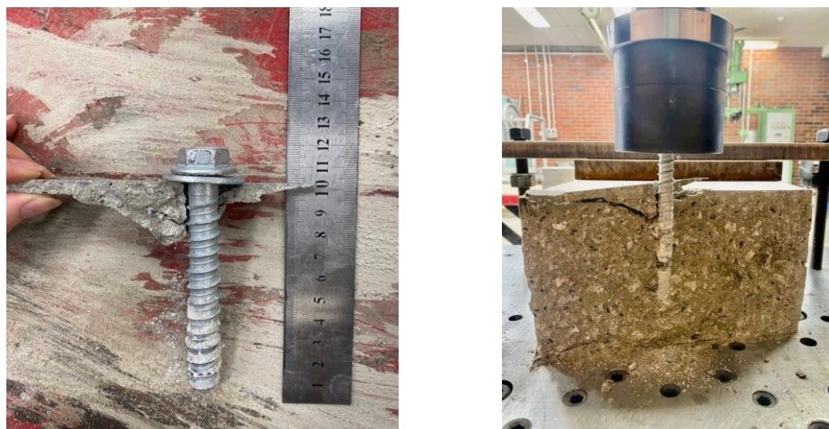
Fig. 7. Representative Combined Failure (B2-28-90)
