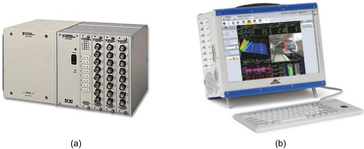
Fig. 5. Multi-channel dynamic measuring devices used in the experiment a) NI SCXI-1000DC measuring device; b) DEWE-3020 measuring device (The images were taken from the user manuals provided by the manufacturers of the measuring equipment)
