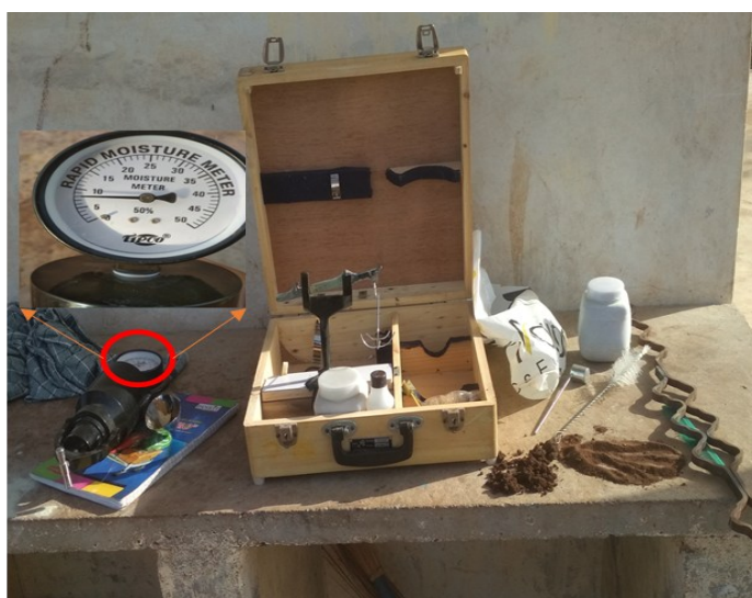
Fig. 5. Rapid moisture meter used to identify soil moisture for moisture movement in experimental box
