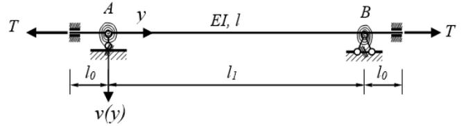
**Fig. 2.** Equivalent model of cable with rotational restraints
