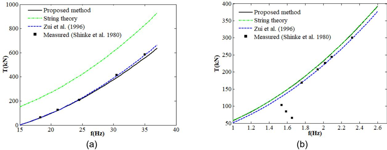
**Fig. 5.** Tension forces: (a) 3.4 m-long cable; (b) 31.5 m-long cable
