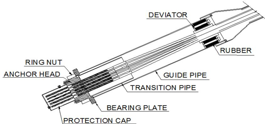
Fig. 8. Stay anchorage configuration with elastic support, rubbers, of An Dong extradosed Bridge
