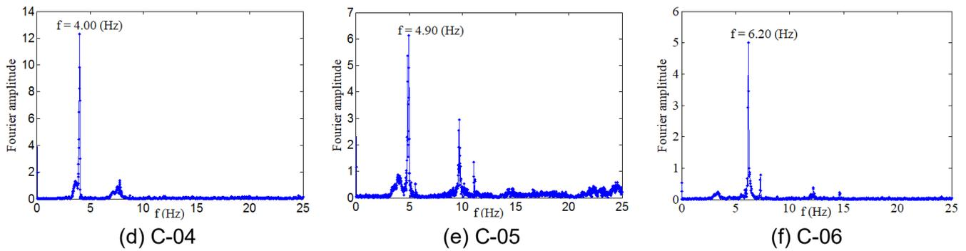
**Fig. 9.** Power spectra of response of six selected cables
