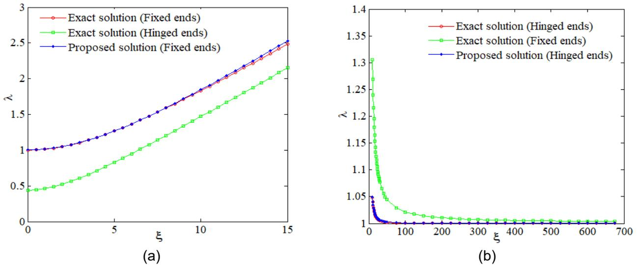
**Fig. 4.** Ratio of fundamental frequency versus  $\xi$ : (a) small  $\xi$ ; (b) large  $\xi$
