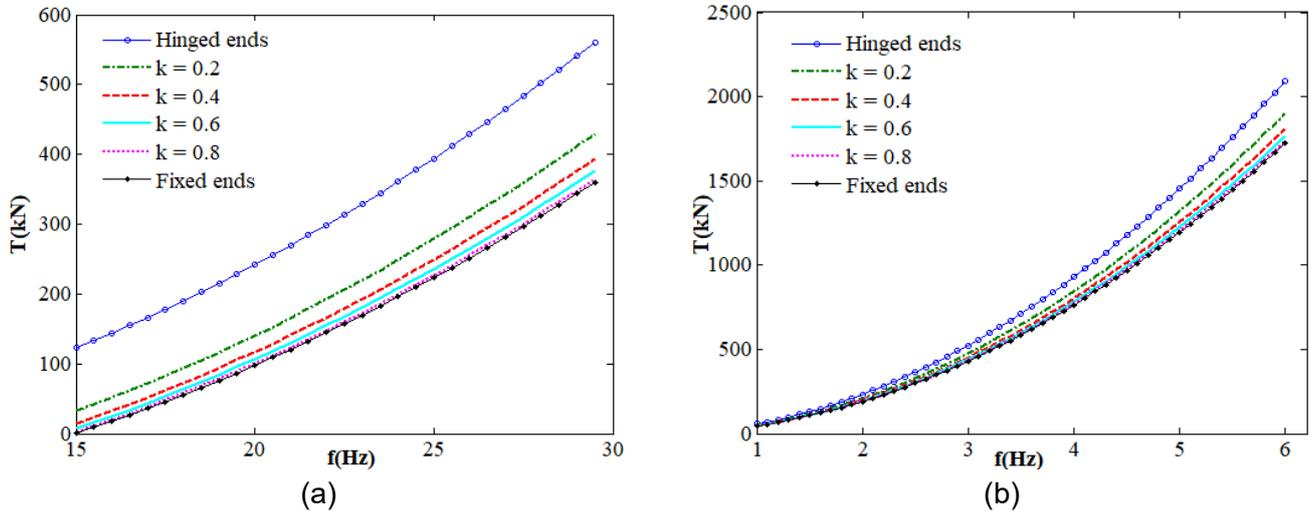
**Fig. 6.** Impact of boundary conditions on cable tension: (a) small  $\xi$ ; (b) large  $\xi$
