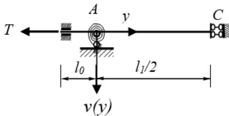
**Fig. 3.** Half taut-string cable model with a spring
