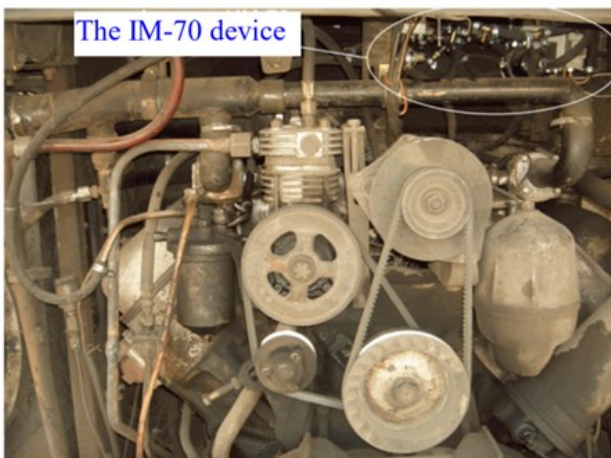
Fig 7. Installation of IM-70 device in the bus engine
