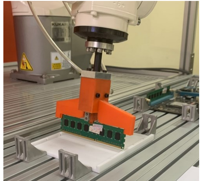
Figure 8. Tilt angle b of the gripper when picking up RAM modules
