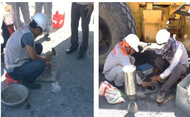
Figure 4. Checking density by sand cone method
