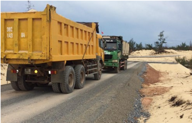
Figure 6. Trafficking test of the trial unpaved road
