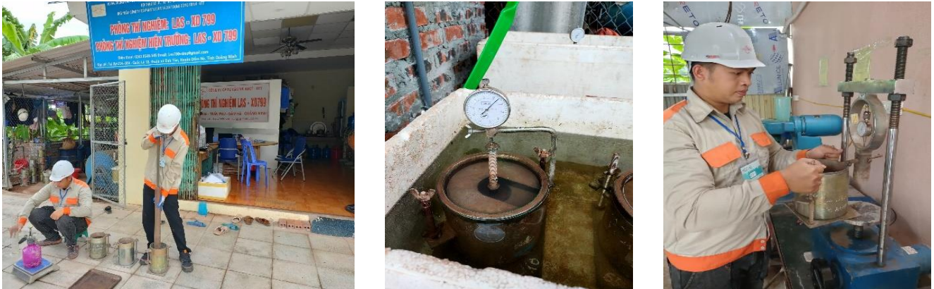
Fig 3. Testing work of California Bearing Ratio (CBR) of Laboratory-Compacted Soils
