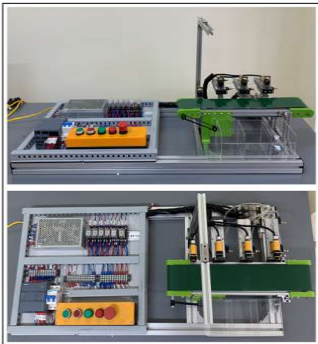
Figure 2. Model of defective product sorting system
